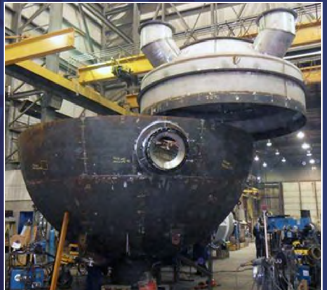
Installing Plenum into Vessel Head
